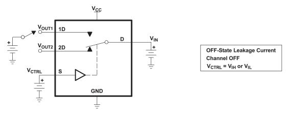
Figure 13. OFF-State Leakage Current
