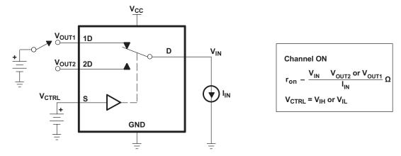
Figure 12. ON-State Resistance (r<sub>on</sub>)
