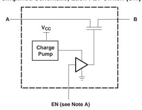
EN is the internal enable signal applied to the switch.
