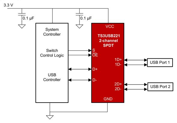
Figure 15. Simplified Schematic
