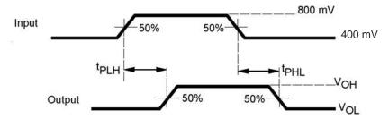
Figure 10. Propagation Delay
